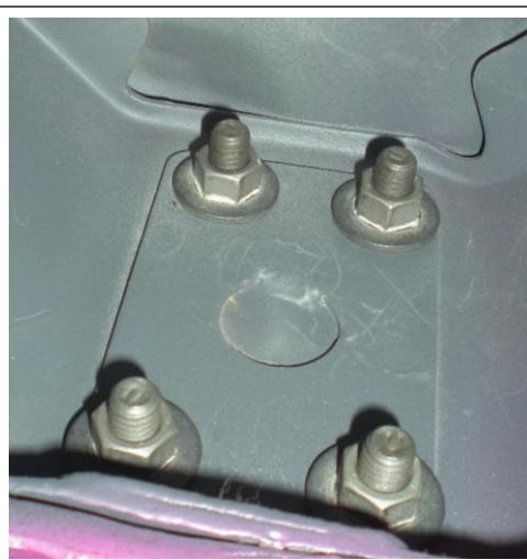
1970 440 + 6 or Hemi reference reinforcement plate inside of the rear torque box
