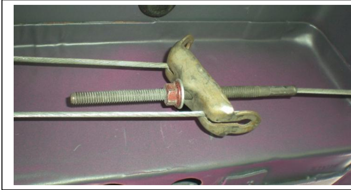
1970 Emergency brake adjuster. The bracket should be zinc plated and the adjusting nut should be plated red zinc dichromate.
