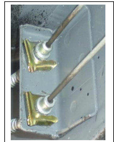
The retaining clips should be phosphate plated .
