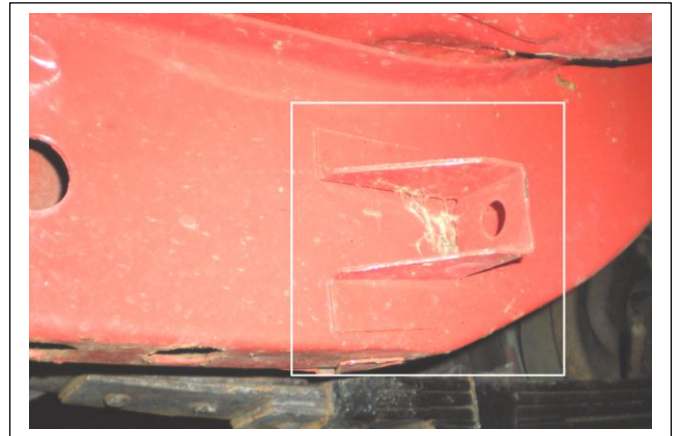
Parking brake cable support bracket position starting in 1971 on right hand frame rail
