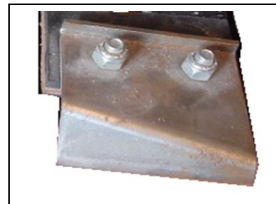
Aftermarket hanger back side. As you can tell rivets are not used.
